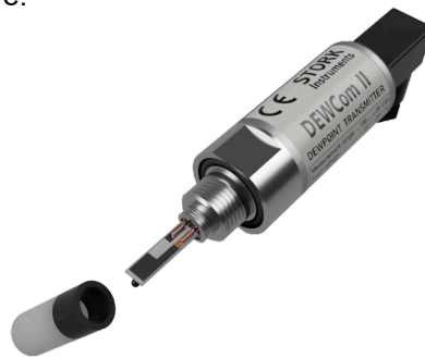
Figure 20. Replacement of filter
