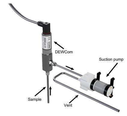
6. Arrangement for measurement in static system such as glove boxes. Always mount the sensor near outlet of glove box
